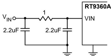
Figure 1. C-R-C filter used to reduce input ripple
