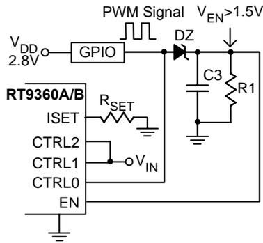
Figure 7. The GPIO PWM dimming application circuit
