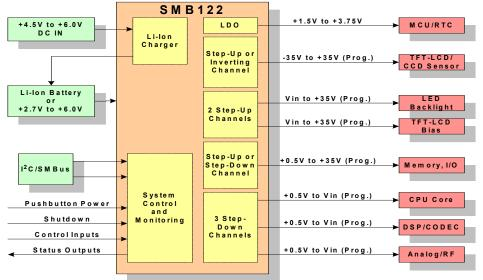
Figure 1 – Applications block diagram featuring the SMB122 eight-channel, programmable DC/DC converter. This integrated power supply and battery manager provides precision regulation, monitoring, cascade sequencing, output margining and battery charging.
