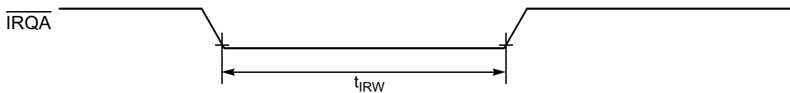
Figure 10-6 External Interrupt Timing (Negative Edge-Sensitive)
