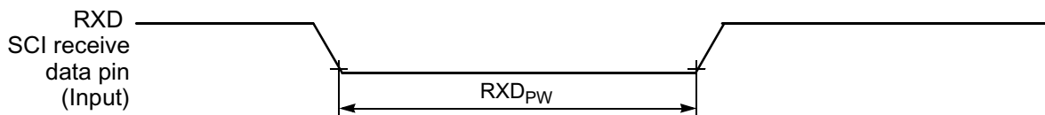
Figure 10-15 RXD Pulse Width
