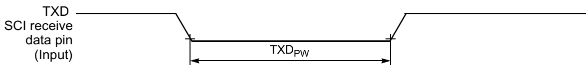
Figure 10-16 TXD Pulse Width
