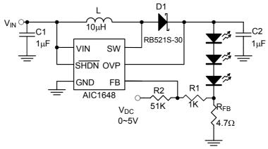
Fig. 18 Dimming Control Using a DC Voltage
