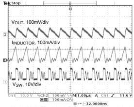
$V_{IN}$ =3.6V; 3 LEDs; L1=10 $\mu$ F; C<sub>OUT</sub>=0.22 $\mu$ F; I<sub>LED</sub>=20mA Fig. 12 Start-Up from Shutdown
