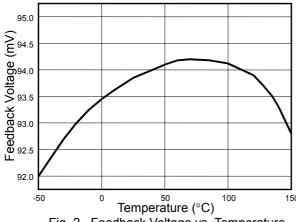
Fig. 2 Feedback Voltage vs. Temperature
