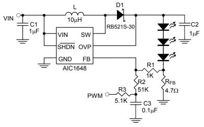
Fig. 19 Dimming Control Using a Filter PWM Signal
