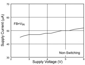
Fig. 4 Supply Current vs. Supply Voltage
