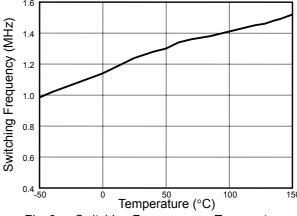
Switching Frequency vs. Temperature Fig. 3
