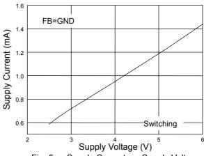
Supply Current vs. Supply Voltage Fig. 5
