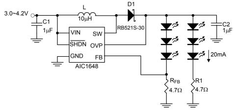
Fig. 20 Six White LEDs Application in Li-lon Battery
