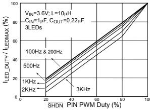
Dimming Control by Shutdown PIN Fig. 7
