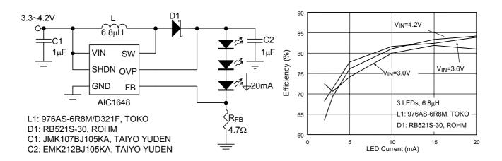
Fig. 1 Li-lon Powered Driver for Three White LEDs
