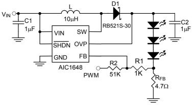
Fig. 17 Dimming Control Using a PWM Signal
