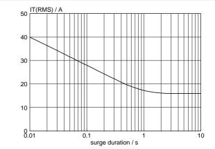
Fig.5. Maximum permissible repetitive rms on-state current  $I_{T(RMS)}$ , versus surge duration, for sinusoidal currents, f = 50 Hz;  $T_{hs} \le 38$  °C.
