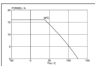
Fig.4. Maximum permissible rms current  $I_{\text{T(RMS)}}$ , versus heatsink temperature  $T_{\text{hs}}$ .
