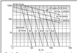
Fig.12. Typical commutation dV/dt versus junction temperature, parameter commutation dl<sub>T</sub>/dt. The triac should commutate when the dV/dt is below the value on the appropriate curve for pre-commutation  $dI_{\tau}/dt$ .
