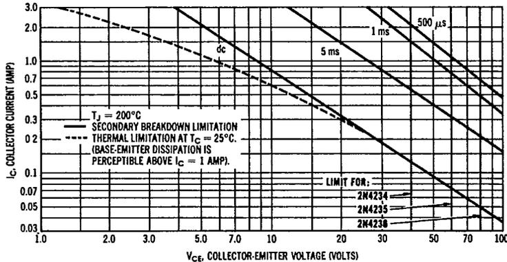
The Safe Operating Area Curves indicate  $I_C - V_{CE}$  limits below which the device will not enter secondary breakdown. Collector load lines for specific circuits must fall within the applicable Safe Area to avoid causing a catastrophic failure. To insure operation below the maximum  $T_J$ , power-temperature derating must be observed for both steady state and pulse power conditions.
