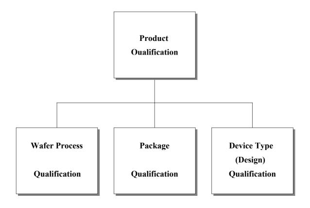
All product qualifications are split into three distinct steps as shown above. This same procedure is also used to qualify a change. Before a product is released for use, it must have been manufactured using a qualified wafer and package process. Before a device is released for production processing, it must also have successfully completed its required specific qualification.
