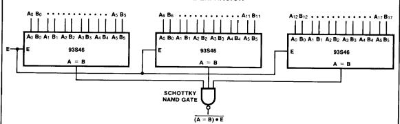
NOTE: This method of expansion adds one gate delay (~3 ns) to the '46, independent of the word length that is compared.
