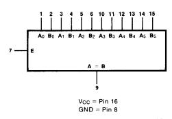
**FUNCTIONAL DESCRIPTION** — The '46 is a very high speed 6-bit identity comparator. The A = B output is HIGH when the Enable (E) is HIGH and the two 6-bit words are equal. Equality is determined by Exclusive-NOR circuits which individually compare the equivalent bits from each word. When any two of the equivalent bits from each word have different logic levels, the A = B output is LOW.
