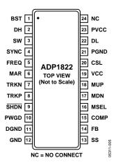
Figure 4. Pin Configuration
