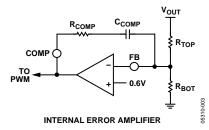
Figure 19. Compensation Using the ESR Zero
