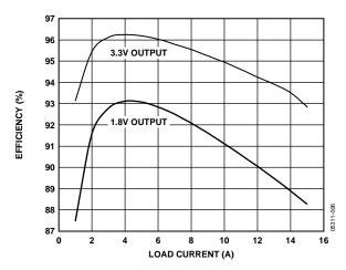
Figure 2. Efficiency vs. Load Current, 5 V Input
