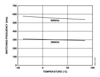
Figure 9. Switching Frequency vs. Temperature
