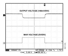
Figure 16. Output Voltage Margin-Down Response
