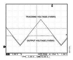
Figure 18. Output Voltage Tracking Response
