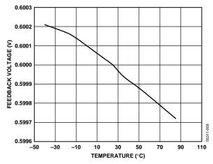
Figure 8. FB Regulation Voltage vs. Temperature
