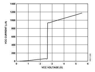
Figure 7.  $V_{\text{DD}}$  Supply Current vs. Voltage
