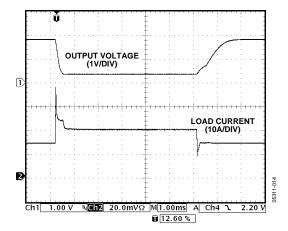
Figure 13. Output Short-Circuit Response and Recovery
