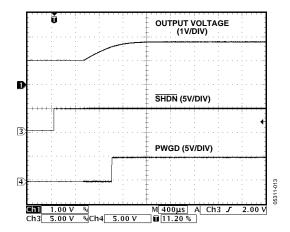
Figure 12. Power-On Response, Prebiased Output
