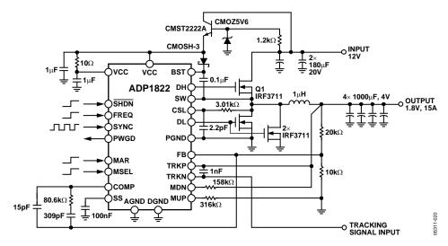
Figure 22. Typical Application Circuit, 12 V Input
