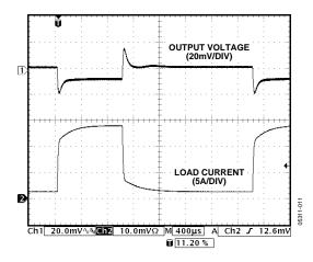
Figure 10. Load Transient Response, 1.5 A to 15 A
