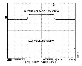
Figure 17. Output Voltage Margin-Up Response
