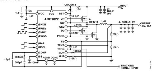
Figure 21. Typical Application Circuit, 5 V Input
