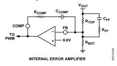
Figure 20. Compensation Using Feed-Forward
