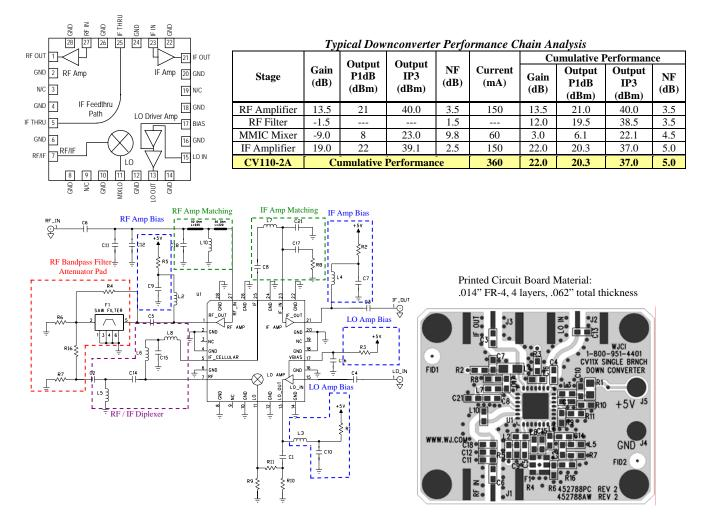
**CV110-2A**: The application circuit can be broken up into four main functions as denoted in the colored dotted areas above: RF/IF diplexing (purple), amplifier matching (green), filtering (red), and dc biasing (blue). There are various placeholders for chip components in the circuit schematic so that a common PCB can be used for all WJ single-branch converters. Additional placeholders for other optional functions such as filtering are also included.
