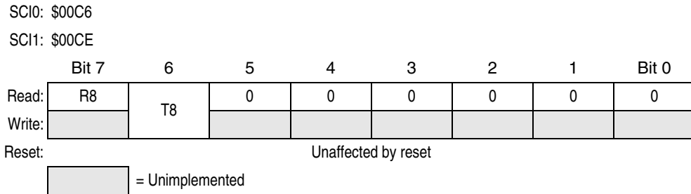
Figure 14-23. SCI Data Register High (SC0DRH or SC1DRH)
