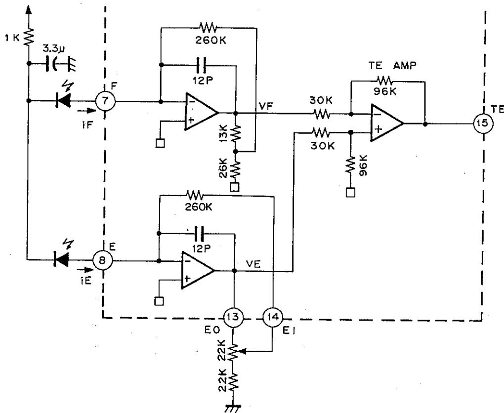
The difference between  $V_E$  and  $V_F$  is obtained at the tracking error amplifier. This amplifier output is the current difference between photo diodes E and F converted into voltage output.
