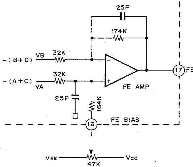
$$\begin{aligned} \text{FE output voltage (low frequency) turns to } V_{\text{FE}} &= 5.4 \times (V_A - V_B) \\ &= (iPD2 - iPD1) \times 315\text{k}\Omega. \end{aligned}$$
