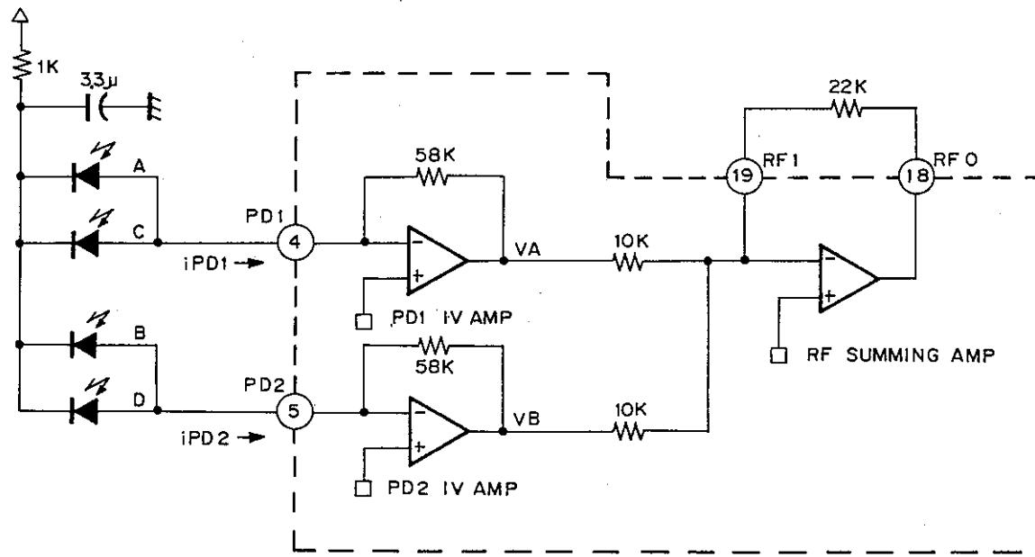
$$\begin{aligned} \text{RFO output voltage low frequency turns to } V_{\text{RFO}} &= 2.2 \times (V_A + V_B) \\ &= 127.6\text{k}\Omega \times (iPD1 + iPD2). \end{aligned}$$
