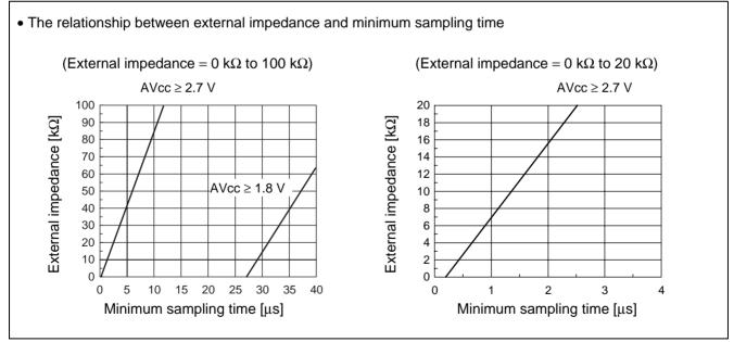
• If the sampling time cannot be sufficient, connect a capacitor of about 0.1 µF to the analog input pin.
