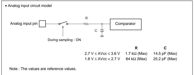
• To satisfy the A/D conversion precision standard, consider the relationship between the external impedance and minimum sampling time and either adjust the resistor value and operating frequency or decrease the external impedance so that the sampling time is longer than the minimum value.
