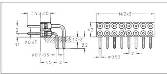
832-10-xxx-20-001 832-90-xxx-20-001 Right angle pin connector: solder tail, double row
