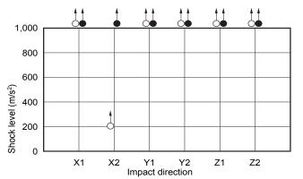
Shock duration: 111 ms, half-sine wave Test condition: coil, energized and de-energized Impact direction: see drawing below Detection level: generation of 1ms or longer contact opening
