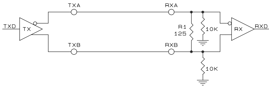
Figure 20. Typical V.11 Interface (Termination Resistor, R1, is Optional.)
