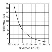
Fig.6 Thermistor curve
