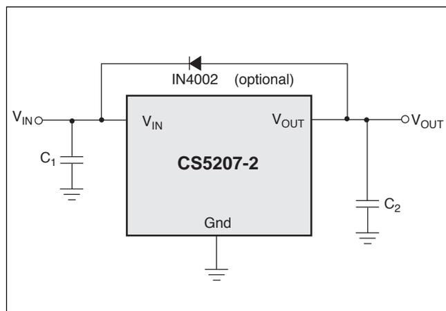
Figure 1. Protection diode scheme for fixed output regulators.
