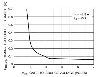
Figure 4. On-Resistance vs. Gate-to-Source Voltage
