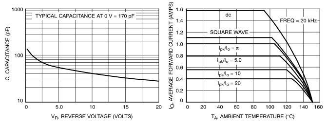
Figure 19. Typical Capacitance
