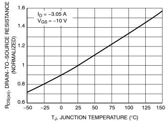
Figure 6. On Resistance Variation with Temperature
