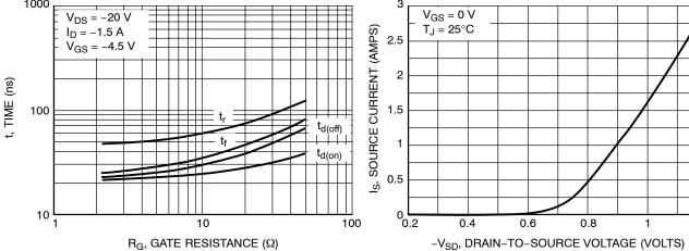
Figure 11. Resistive Switching Time Variation vs. Gate Resistance
