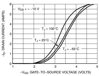
Figure 2. Transfer Characteristics
