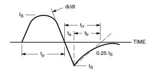
Figure 13. Diode Reverse Recovery Waveform
