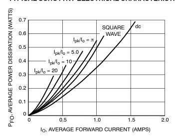
Figure 21. Forward Power Dissipation
