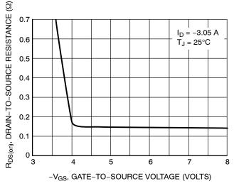
Figure 3. On-Resistance vs. Gate-to-Source Voltage
