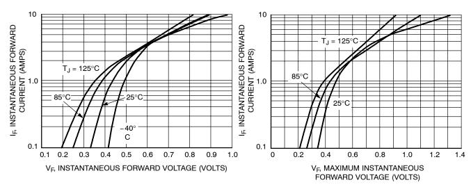
Figure 15. Typical Forward Voltage
