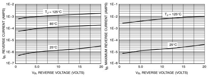
Figure 17. Typical Reverse Current
