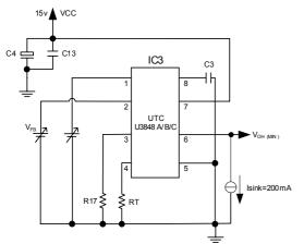
FIG.10 driver test circuit with sink current
