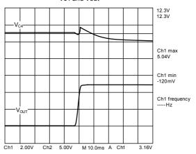
Startup Behavior At Nominal Load Condition  $V_{DCIN}$ =120 V
