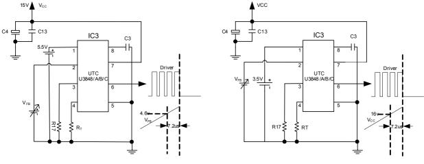
FIG.8 OLP test circuit
