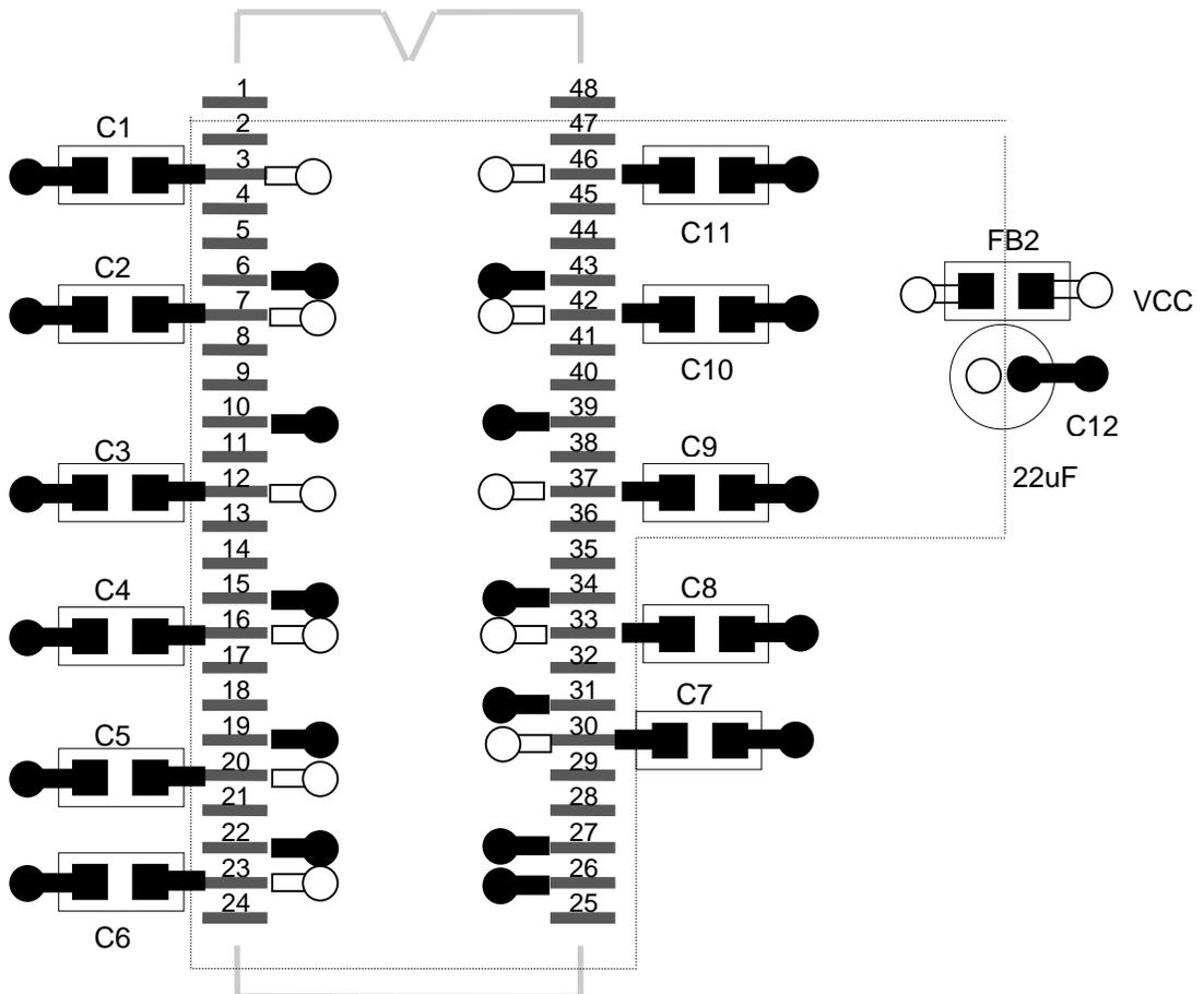
This is only a layout recommendation for best performance and lower EMI. the designer may choose a different approach but C1, C2, C3, C4, C5, C6, C7, C8, C9, C10, and C11 (all are 0.1 uf) should always be used and placed as close to their VDD pins as is physically possible.
