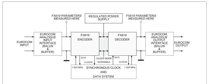
Fig.2 Eurocom System Configuration – showing the FX619, which with the indicated interfacing, will conform to the Eurocom Basic Parameters Specification D1 – IA8.
