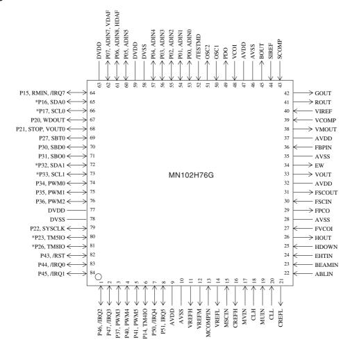
QFP084-P-1818E \*Lead-free \*5 V dielectric Nch open drain output pin
