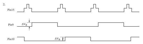
Input 100 % white signal and adjust the voltage of Pin4 so that  $\Delta V_B$  becomes 0 mV. Let the adjusted voltage be  $V_{AD4}$ .
