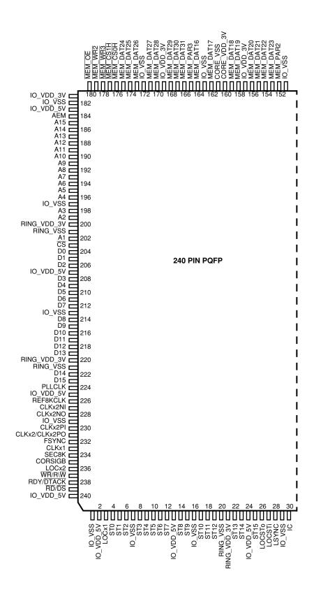
**Figure 2. Pin Connections**
