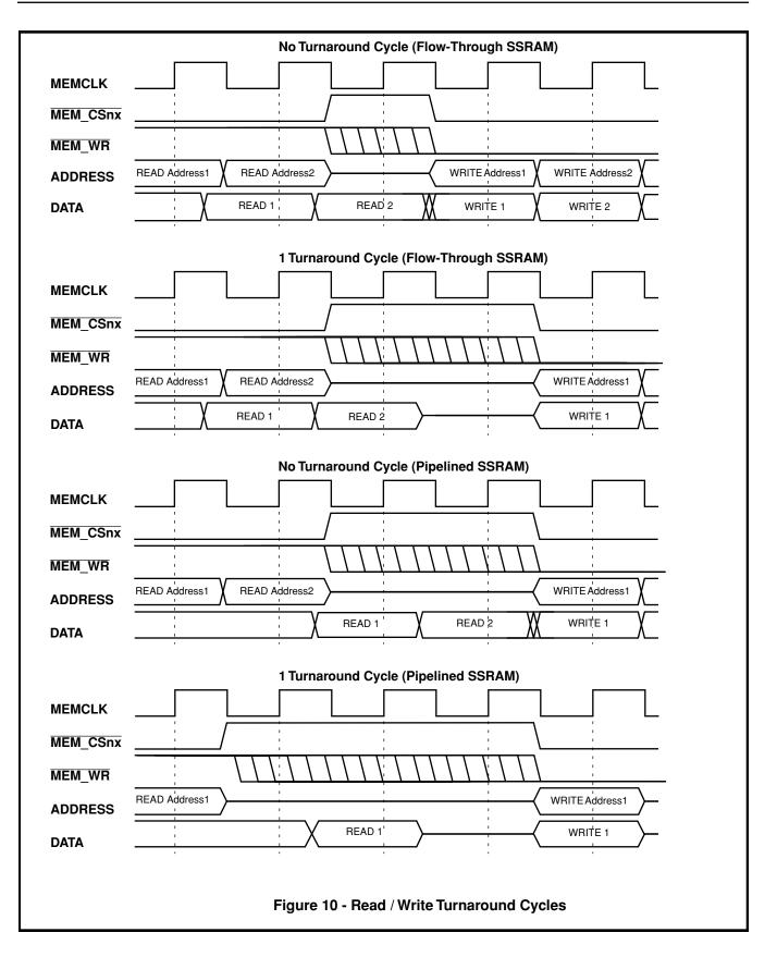
It should be noted that turnaround cycles, in effect, restrict the memory bandwidth, and therefore the operation of the MT90500. Maximum throughput is achieved with full clock speed on the MCLK input (which drives MEMCLK), and with non-pipelined synchronous SRAM without turnaround cycles (easiest achieved by using a
