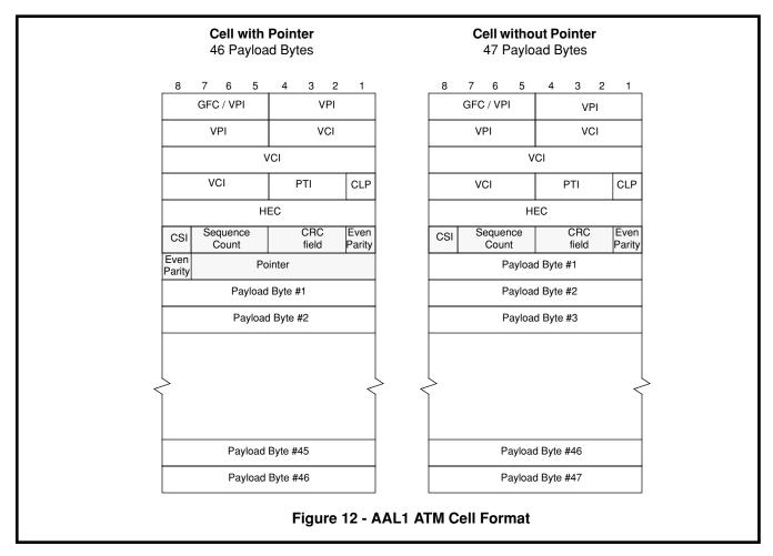
n =1; and over partially-filled cells (where n is less than, or equal to, the payload size). The cell parameters are configured through the microprocessor port. Figure 12 gives examples of the ATM AAL1 cell formats.
