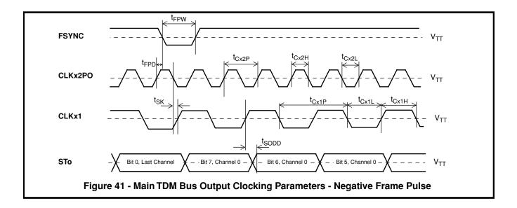
NOTE: Some SCSA devices may require a wider frame pulse at 4 Mbps and at 8 Mbps than the MT90500 provides. Also, H-MVIP uses a 488 ns wide frame pulse at 8 Mbps.
