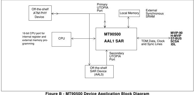
Figure B - MT90500 Device Application Block Diagram
