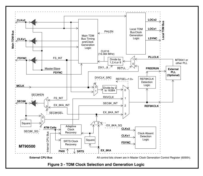
The CLKx2 signal can be selected as single-ended or differential. (Differential CLKx2 allows compatibility with the H-MVIP bus.) In TDM Timing Slave, the CLKx2 signal can be input on the CLKx2 pin, or the differential CLKx2PI and CLKx2NI pins. This selection is made with CLKTYPE in the TDM Bus Type Register at address 6010h. In TDM Timing Master, the CLKx2 signal is output on the CLKx2/CLKx2PO pin, and an inverted clock is available on the CLKx2NO pin.
