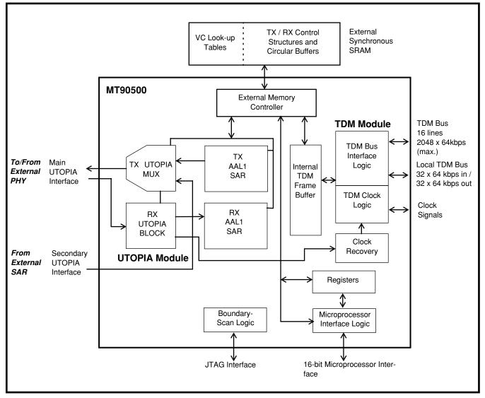
Figure 1 - MT90500 Block Diagram
