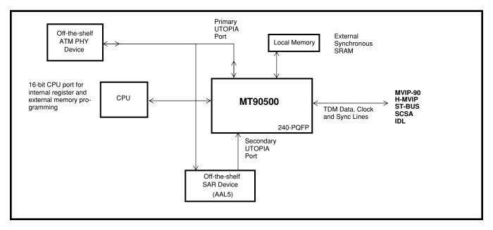
Figure 62 - MT90500 Device Application Block Diagram
