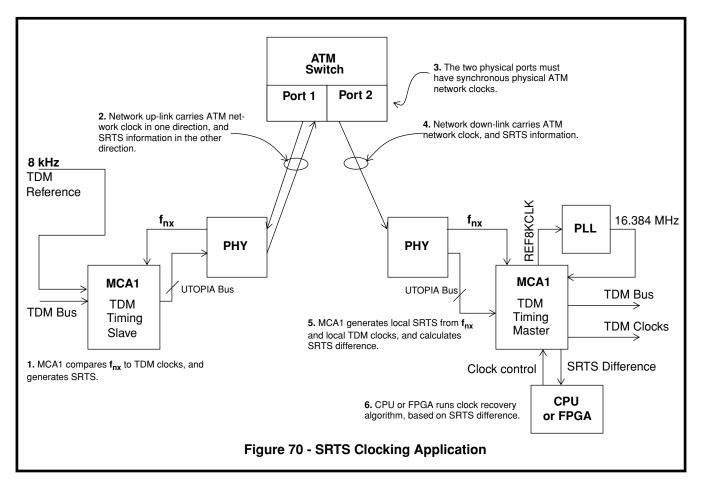
Another consideration in the application of SRTS clock recovery using the MT90500 is the 5 RTS buffer in the Receive SRTS circuitry. This puts an upper limit on the CDV (Cell Delay Variation) of the receive VC carrying SRTS. Each RTS in the 5 RTS buffer is carried by one 8 cell sequence, and thus represents a fixed amount of time dependent on the number of TDM channels being carried. Table 102 summarizes the maximum CDV supported by the Receive SRTS circuitry at various numbers of TDM channels.
