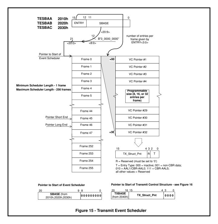
When the MT90500 is used to transmit CBR-AAL5 cells, additional register programming is required to properly initialize the TX\_SAR and the schedulers to send cells containing 32-bit CRCs. Regardless of which scheduler(s) is (are) to be used for transmission of the ATM cells, the following initialization settings must be made:
