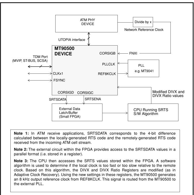
Figure 36 - Clock Recovery Using SRTS Method (CPU)
