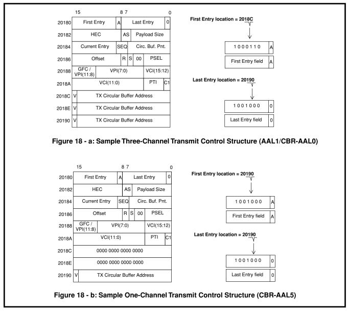
bits are one-hot bits which represent cells with sequence numbers 0, 2, 4, and 6, respectively - see Table 10 below for an explanation of bit operation). The MT90500 also supports proprietary pointer transmissions in which a P-byte is sent every 4 cells (PSEL = A hex) or every other cell (PSEL = F hex). Using these proprietary methods, up to 122 channels can be sent on a particular VC, but this is only possible if the receiving chip can handle the extra P-bytes during a cycle.
