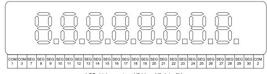
LCD driving system 1/2 bias, 1/3 duty, 3V
