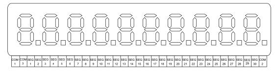
LCD driving system 1/2 bias, 1/3 duty, 3V
