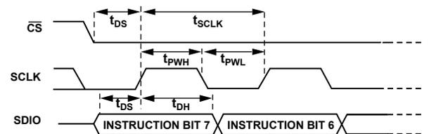
Figure 11. Timing Diagram for Register Write to AD9725
