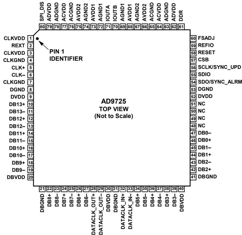
Figure 4. Pin Configuration
