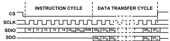
Figure 10. Serial Register Interface Timing LSB First
