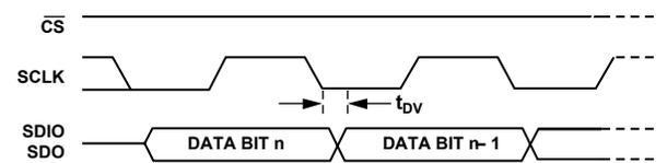
Figure 12. Timing Diagram for Register READ to AD9725
