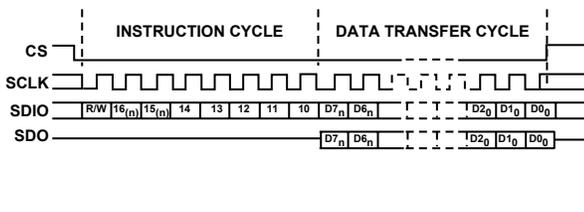
Figure 9. Serial Register Interface Timing MSB First
