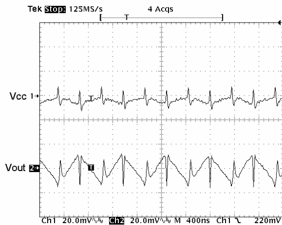
Figure 14. 1.5x Mode Operating Waveforms
