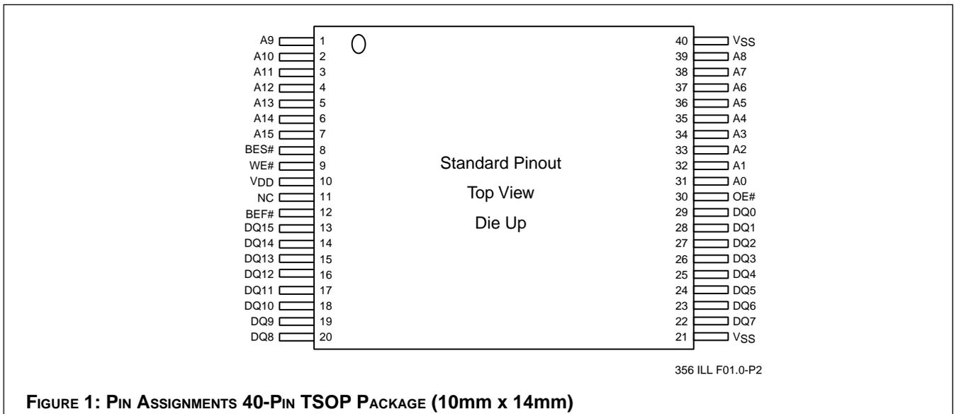
**FIGURE 1: PIN ASSIGNMENTS 40-PIN TSOP PACKAGE (10mm x 14mm)**
