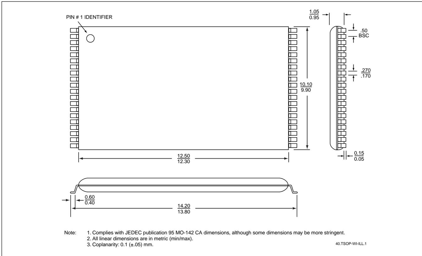
**40-PIN THIN SMALL OUTLINE PACKAGE (TSOP) 10MM X 14MM**
