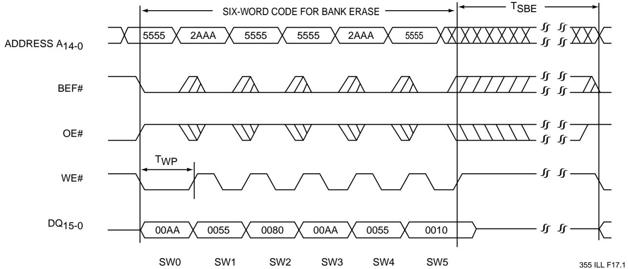
Note: The device also supports BEF# controlled Bank Erase operation. The WE# and BEF# signals are interchangeable as long as minimum timings are met. (See table 10)
