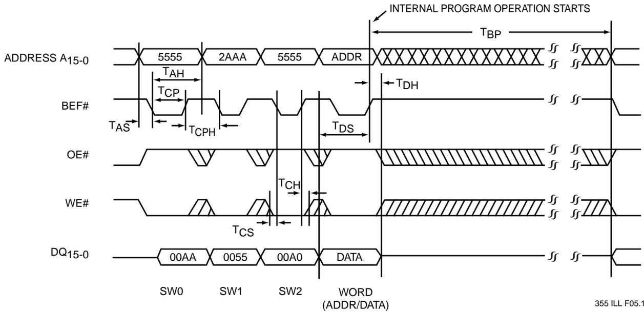
FIGURE 6: BEF# CONTROLLED PROGRAM CYCLE TIMING DIAGRAM
