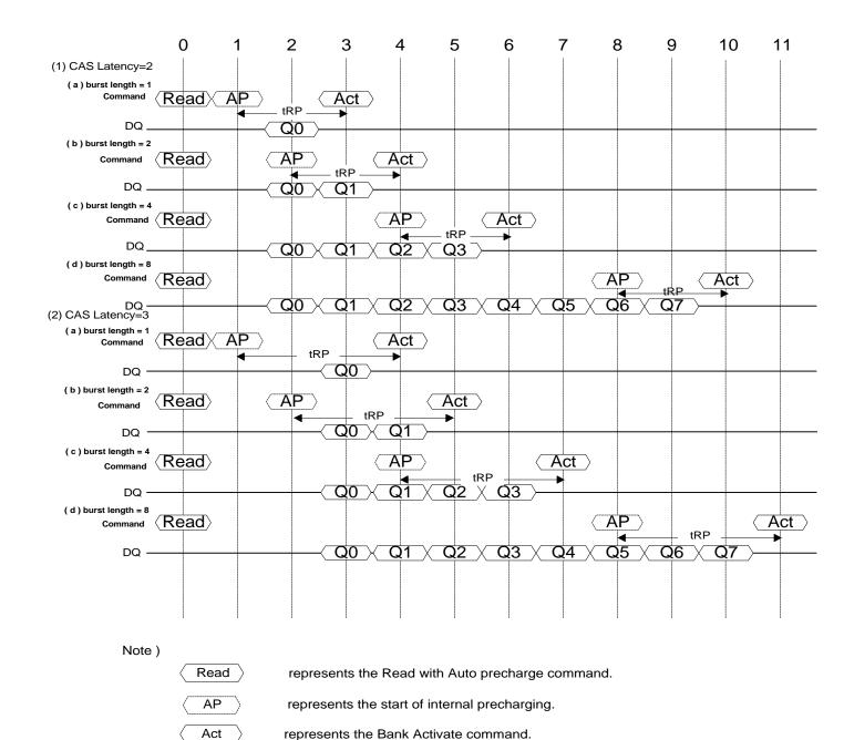
When the Auto precharge command is asserted, the period from Bank Activate command to the start of internal precgarging must be at least tRAS(min).
