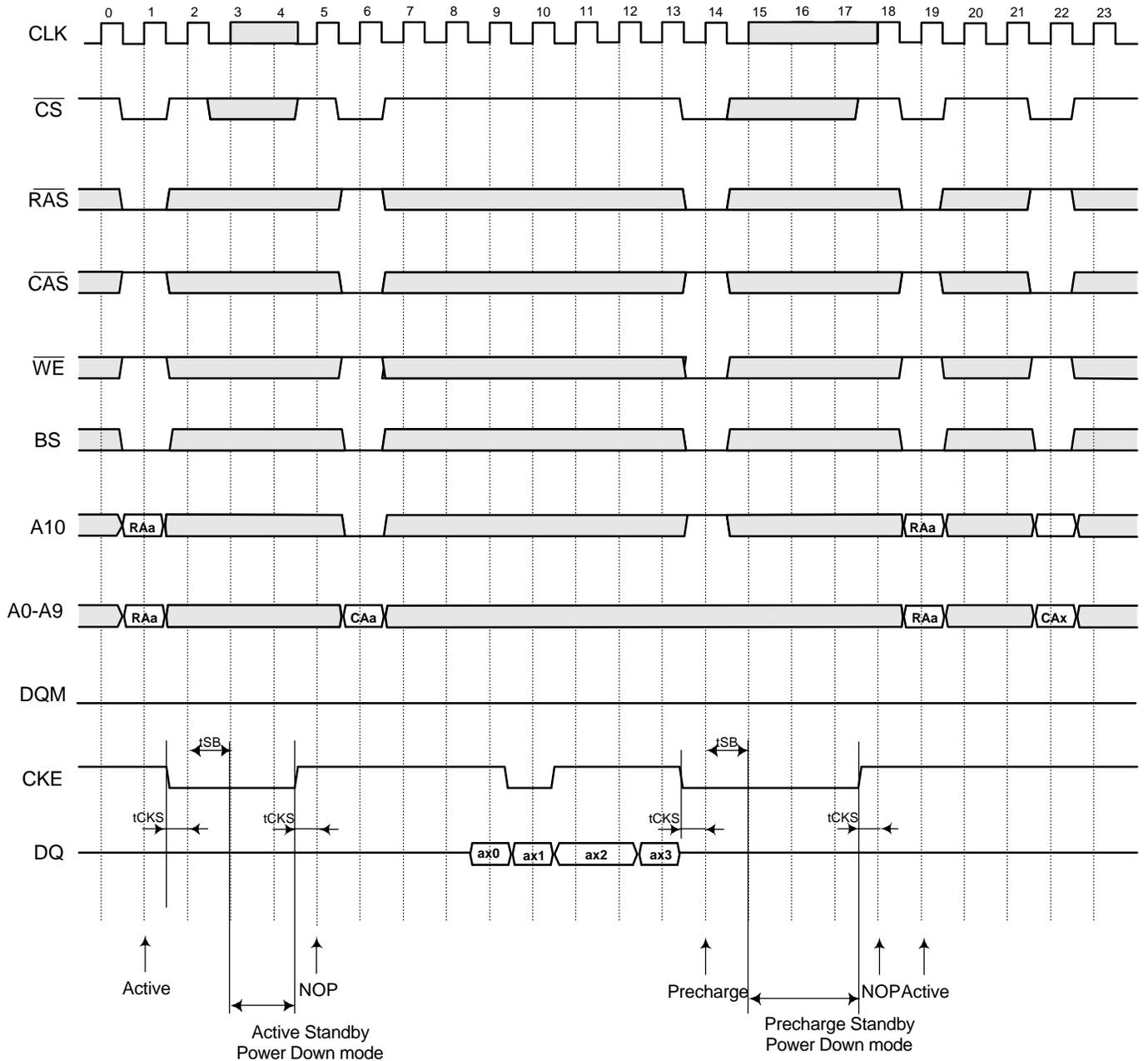
Note: The PowerDown Mode is entered by asserting CKE "low".
