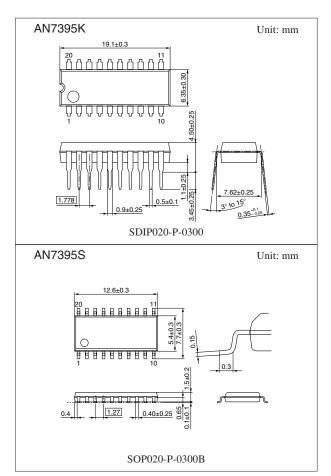
Note) The packages (SDIP020-P-0300 and SOP020-P-0300B) of this product will be changed to lead-free type (SDIP020-P-0300A and SOP020-P-0300E). See the new package dimensions section later of this datasheet.
