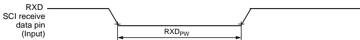
Figure 25. RXD Pulse Width
