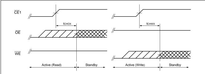
Note: Both  $t_{CHOX}$  and  $t_{CHWX}$  define the earliest entry timing for Standby mode. If either of timing is not satisfied, it takes  $t_{RC}$  (Min) period from either last address transition of  $A_2$ ,  $A_1$ , and  $A_0$ , or  $\overline{CE}1$  Low to High transition.
