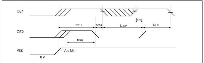
Note : The  $t_{C2HL}$  specifies from CE2 Low to High transition after  $V_{DD}$  reaches specified minimum level.  $\overline{CE1}$  must be brought to High prior to or together with CE2 Low to High transition.
