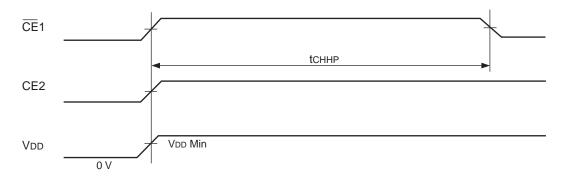
Note : Both  $\overline{\text{CE}}1$  and CE2 must be High together with V<sub>DD</sub>. Otherwise either POWER-UP Timing #1 or #2 must be used for proper operation.
