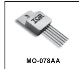
The IRUH50P253B1M is a space qualified, ultra low dropout linear regulator designed specifically for space applications. This product has been characterized to a total ionizing dose of 1.0 Mrad(Si) per MIL-STD-883, Method 1019 at both high and low dose rates under biased and unbiased conditions to account for ELDRS effects in bipolar devices. The ultra low dropout voltage of 0.4V@ 3A makes the part particularly useful for applications requiring low noise and higher efficiency.
