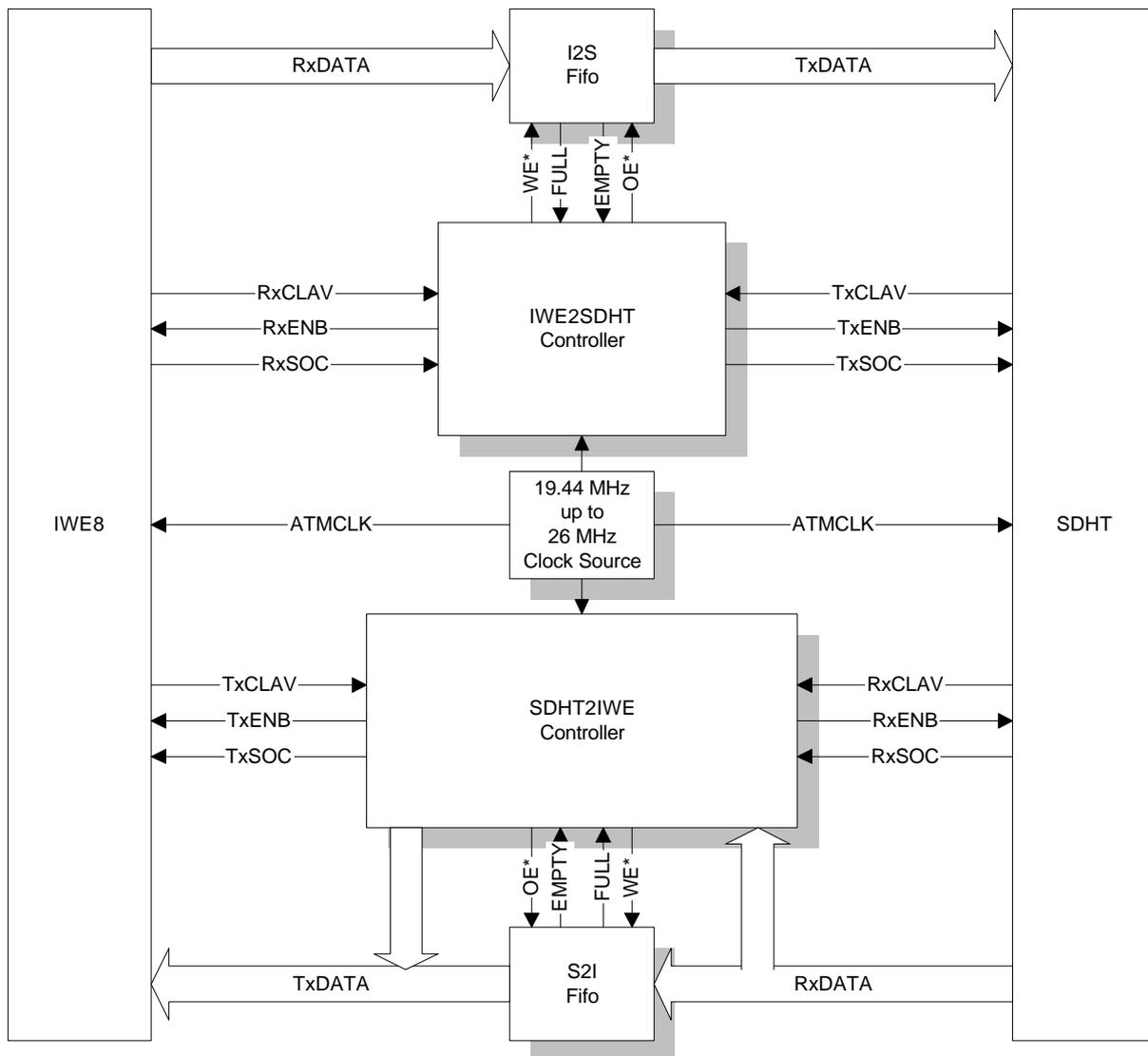
Since both PHYs operate in UTOPIA slave mode, additional logic (shaded in the above block diagram) has to perform the master function. This comprises
