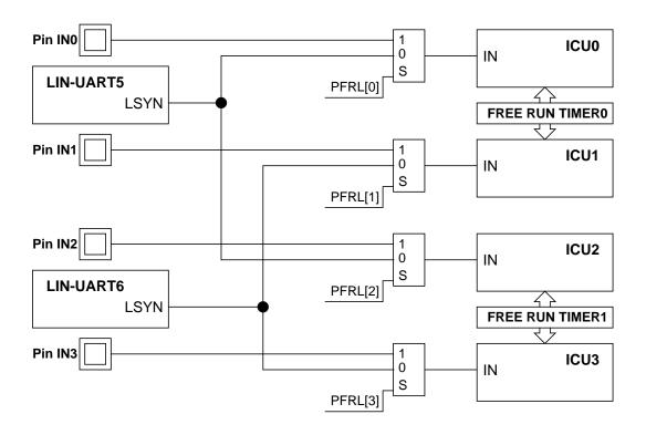
If the PFR bit is set, the ICU is connected to its input pin IN.
