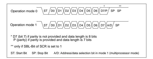
**Note:** If BDS-Bit of the Serial Status Register (SSR) is set to "1", then the bit stream processes as: D7, D6, ..., D1, D0, (P).
