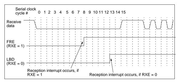
The figure above demonstrates the LIN synch break detection and flag set timing.
