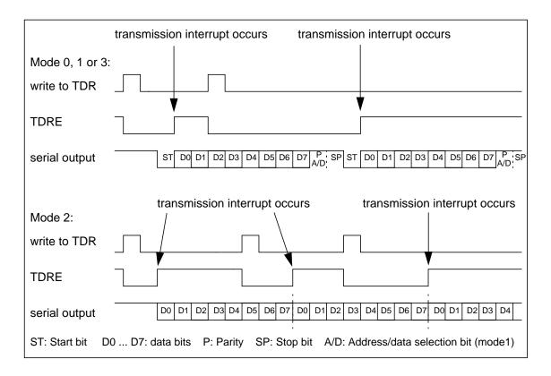
Note: The example above shows not all possible transmission options for mode 0. Here it is: "8p1" (p = "E" or "O"). Parity is not provided in mode 3.
