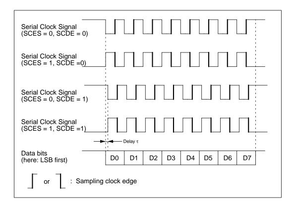
$$\tau = \frac{1}{\phi} \qquad \phi = MCU \text{ clock cycle}$$
