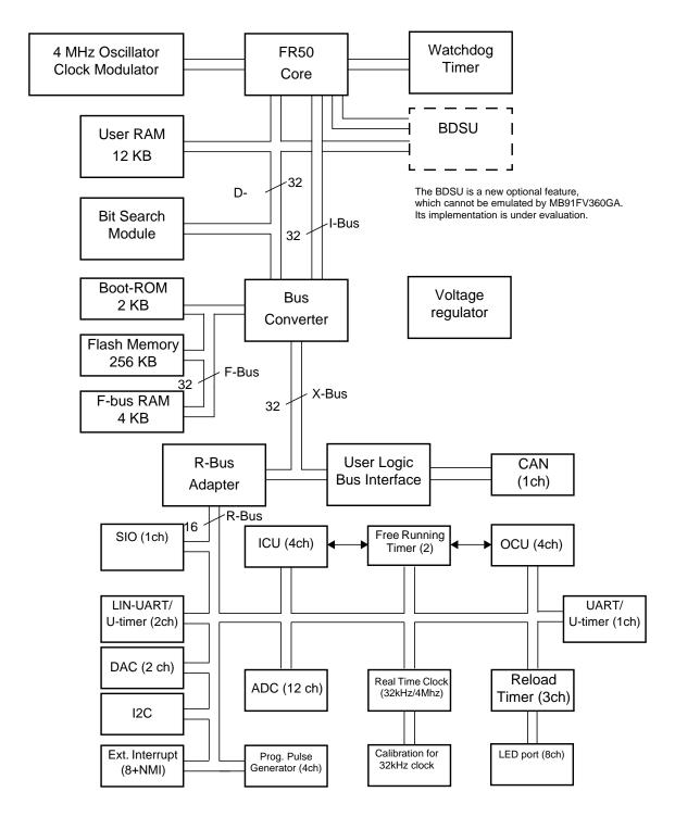
LIN-UART is a new feature which cannot be emulated by MB91FV360GA. The correct functionality cannot be guaranteed until evaluation has been carried out..
