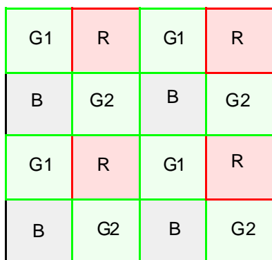
Figure 4. On-chip Bayer CFA
