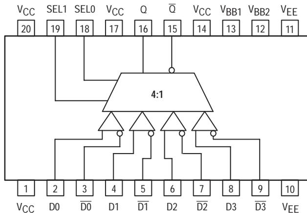
Figure 1. 20-Lead TSSOP (Top View) and Logic Diagram
