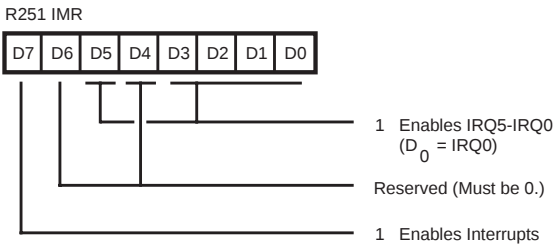
Figure 33. Interrupt Mask Register (FB H : Read/Write)
