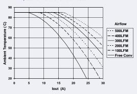
Note A: All data listed in the above graphs has been developed from actual products tested at  $25^{\circ}$ C. This data is considered typical data for the DC-DC Converter. Note B: SOA curves represent operating conditions at which the temperature of the metal case is at or below the maximum specified  $100^{\circ}$ C
