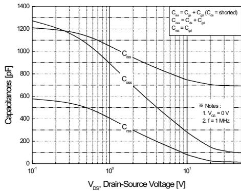
Figure 5. Capacitance Characteristics
