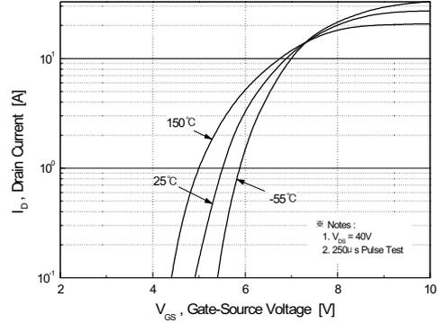
Figure 2. Transfer Characteristics
