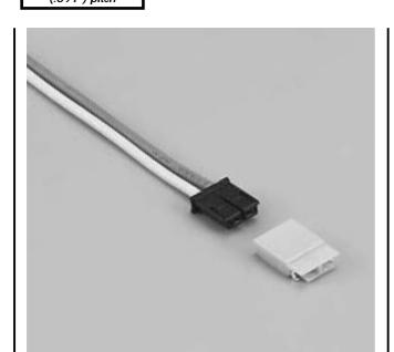
Low profile connector with high withstanding voltage, designed for connecting liquid crystal display backlight lamps to their starters. The BHL connector is 2.8mm (.110") thick, so the mounting height is only 3mm (.118").
