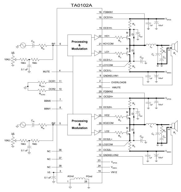
NC - Not Connected (Must Be Left Floating) Note - Heavy Lines Indicate High-Current Paths
