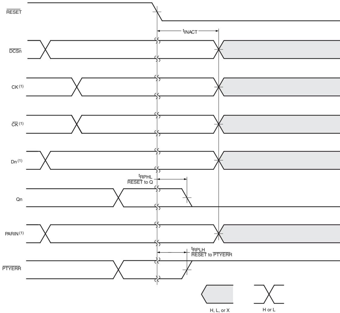
Figure 6 —  $\overline{\text{RESET}}$  switches from H to L
