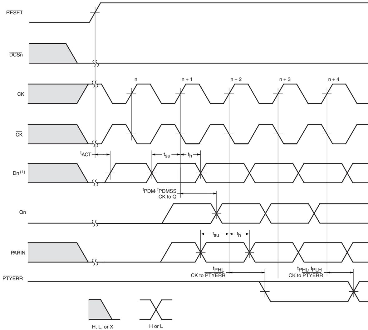
Figure 4 —RESET switches from L to H
