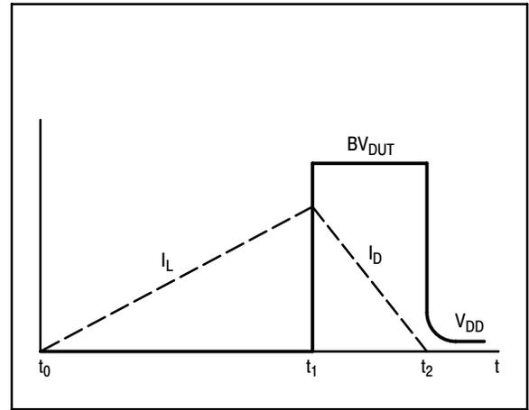
Figure 11. Current-Voltage Waveforms
