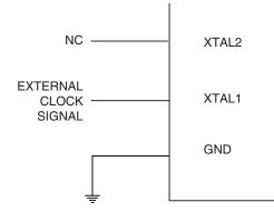
When this clock source is selected, start-up times are determined by the SUT Fuses as shown in Table 7-12.
