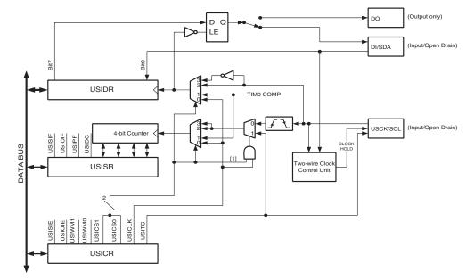
Figure 19-1. Universal Serial Interface, Block Diagram
