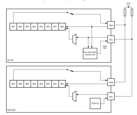
Figure 19-4. Two-wire Mode Operation, Simplified Diagram
