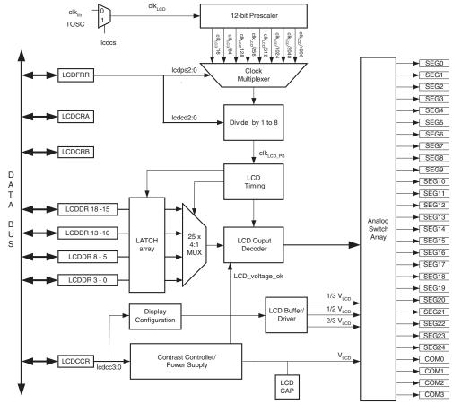
Figure 22-1. LCD Module Block Diagram
