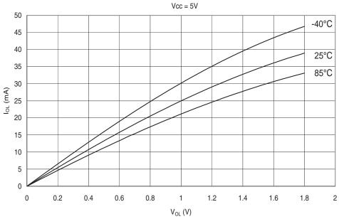
I/O PIN SINK CURRENT vs. OUTPUT VOLTAGE, PORTS A, C, D, E, F, G
