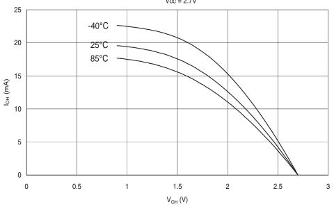
I/O PIN SOURCE CURRENT vs. OUTPUT VOLTAGE, PORTS A, C, D, E, F, G  $V_{CC} = 2.7V$
