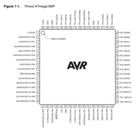
Note: The large center pad underneath the QFN/MLF packages is made of metal and internally connected to GND. It should be soldered or glued to the board to ensure good mechanical stability. If the center pad is left unconnected, the package might loosen from the board.
