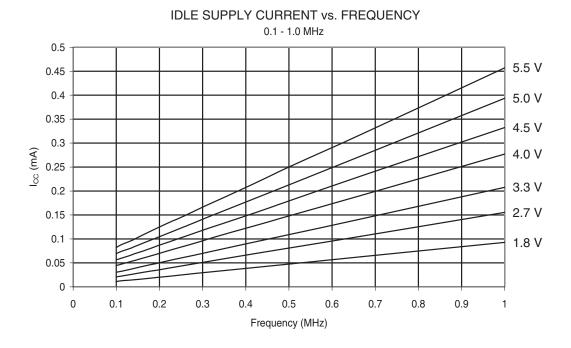
**Figure 28-6.** Idle Supply Current vs. Frequency (0.1 - 1.0 MHz)
