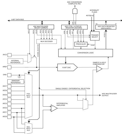
Figure 21-1. Analog to Digital Converter Block Schematic
