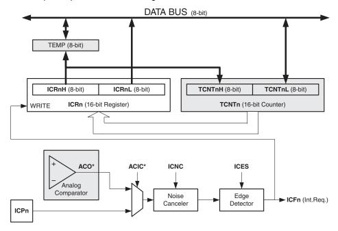
Figure 14-3. Input Capture Unit Block Diagram
