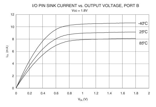
Figure 28-40. I/O Pin Sink Current vs. Output Voltage, Port B (V<sub>CC</sub> = 1.8V)
