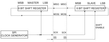
Figure 17-2. SPI Master-slave Interconnection
