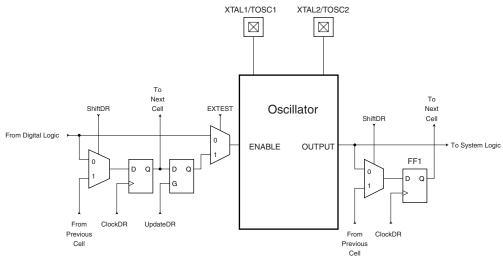
Table 24-1 summaries the scan registers for the external clock pin XTAL1, oscillators with XTAL1/XTAL2 connections as well as 32kHz Timer Oscillator.
