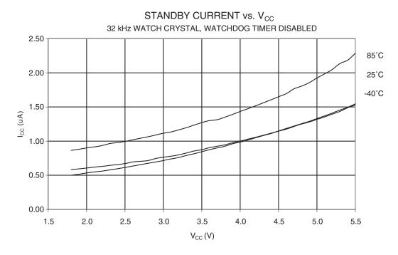
Figure 28-14. Standby Supply Current vs. V<sub>CC</sub> (32 kHz Watch Crystal, Watchdog Timer Disabled)
