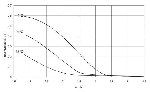
RESET INPUT PIN HYSTERESIS vs. V<sub>CC</sub>
