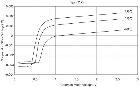
ANALOG COMPARATOR OFFSET VOLTAGE vs. COMMON MODE VOLTAGE
