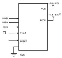
Notes: 1. If the device is clocked by the internal Oscillator, it is no need to connect a clock source to the XTAL1 pin.
