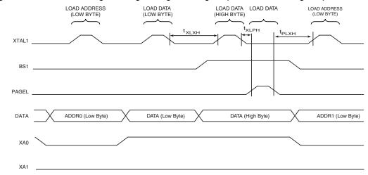
Figure 26-8. Parallel Programming Timing, Loading Sequence with Timing Requirements<sup>(1)</sup>
