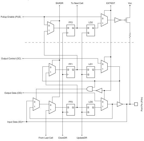
Figure 24-3. Boundary-scan Cell for Bi-directional Port Pin with Pull-up Function.
