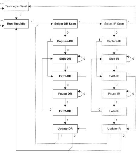
Figure 26-16. State Machine Sequence for Changing/Reading the Data Word
