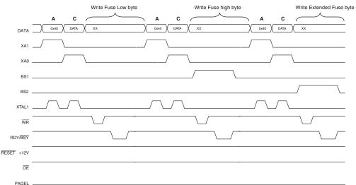
Figure 26-5. Programming the FUSES Waveforms
