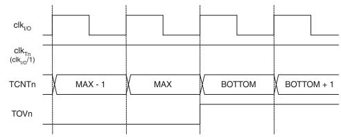
Figure 16-8. Timer/Counter Timing Diagram, no Prescaling
