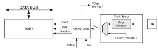
Figure 13-2. Counter Unit Block Diagram
