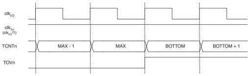
Figure 13-8. Timer/Counter Timing Diagram, no Prescaling
