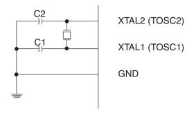
The Oscillator can operate in three different modes, each optimized for a specific frequency range. The operating mode is selected by the fuses CKSEL3:1 as shown in Table 7-5.
