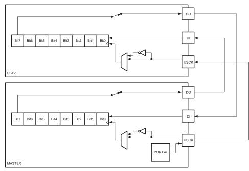
Figure 19-2. Three-wire Mode Operation, Simplified Diagram
