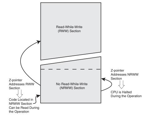
Figure 25-1. Read-While-Write vs. No Read-While-Write
