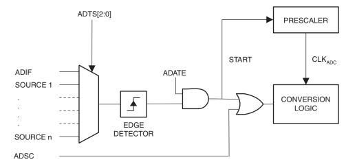
Figure 21-2. ADC Auto Trigger Logic
