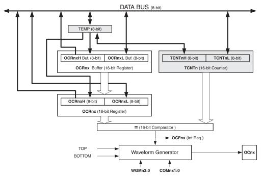
Figure 14-4. Output Compare Unit, Block Diagram
