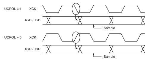
The UCPOLn bit UCRSC selects which XCK clock edge is used for data sampling and which is used for data change. As Figure 18-3 shows, when UCPOLn is zero the data will be changed at rising XCK edge and sampled at falling XCK edge. If UCPOLn is set, the data will be changed at falling XCK edge and sampled at rising XCK edge.
