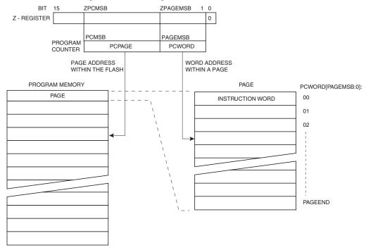
Figure 25-3. Addressing the Flash During SPM<sup>(1)</sup>
