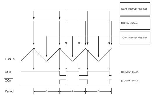
Figure 13-7. Phase Correct PWM Mode, Timing Diagram
