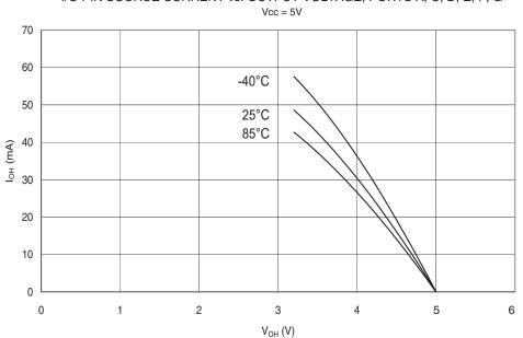
I/O PIN SOURCE CURRENT vs. OUTPUT VOLTAGE, PORTS A, C, D, E, F, G
