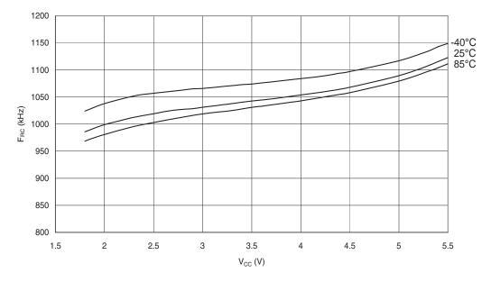
WATCHDOG OSCILLATOR FREQUENCY vs.  $V_{\text{CC}}$
