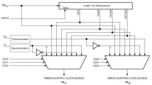
Figure 15-2. Prescaler for Timer/Counter0 and Timer/Counter1<sup>(1)</sup>
