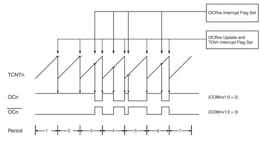
Figure 13-6. Fast PWM Mode, Timing Diagram
