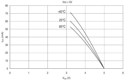
I/O PIN SOURCE CURRENT vs. OUTPUT VOLTAGE, PORT B
