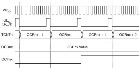
Figure 14-12 shows the count sequence close to TOP in various modes. When using phase and frequency correct PWM mode the OCR1x Register is updated at BOTTOM. The timing diagrams
