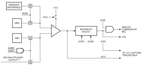
Figure 20-1. Analog Comparator Block Diagram<sup>(2)</sup>
