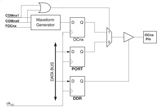
Figure 14-5. Compare Match Output Unit, Schematic
