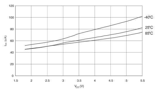
Figure 28-64. Programming Current vs. V<sub>CC</sub>
