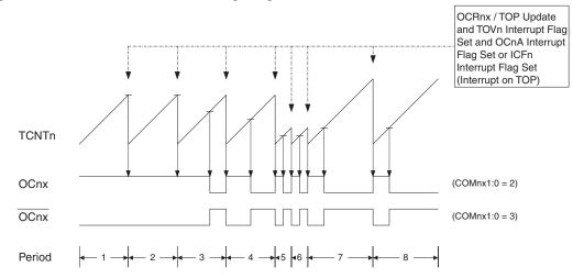
The Timer/Counter Overflow Flag (TOV1) is set each time the counter reaches TOP. In addition the OC1A or ICF1 Flag is set at the same timer clock cycle as TOV1 is set when either OCR1A
