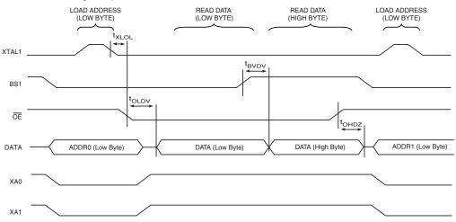
Note: 1. The timing requirements shown in Figure 26-7 (i.e., t<sub>DVXH</sub>, t<sub>XHXL</sub>, and t<sub>XLDX</sub>) also apply to reading operation.
