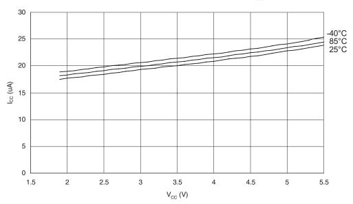
BROWNOUT DETECTOR CURRENT vs. V<sub>CC</sub>
