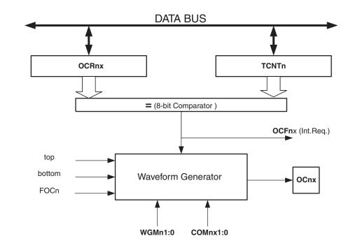
Figure 13-3. Output Compare Unit, Block Diagram
