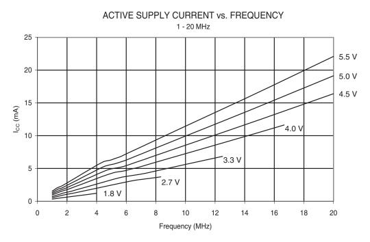
Figure 28-2. Active Supply Current vs. Frequency (1 - 20 MHz)
