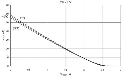
RESET PULL-UP RESISTOR CURRENT vs. RESET PIN VOLTAGE
