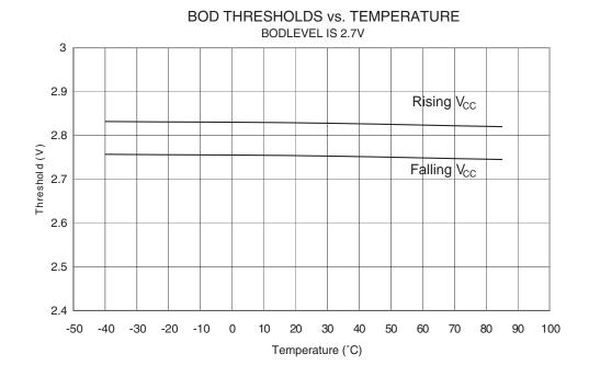
Figure 28-48. BOD Thresholds vs. Temperature (BOD Level is 2.7V)
