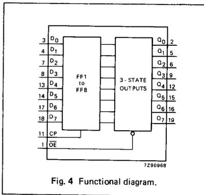
Fig. 4 Functional diagram.
