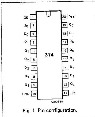
Fig. 1 Pin configuration.
