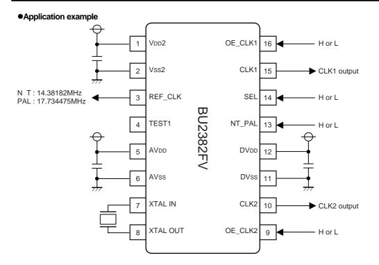
Note) The BU2382FV is basically placed on the board.
