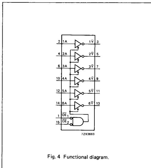
Fig. 4 Functional diagram.
