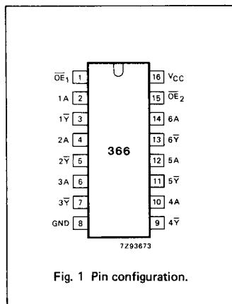
Fig. 1 Pin configuration.
