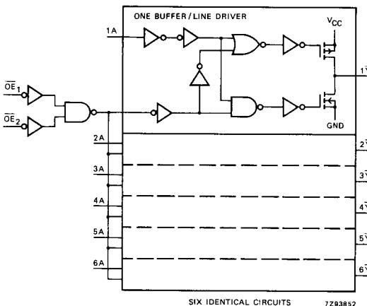
Fig. 5 Logic diagram.
